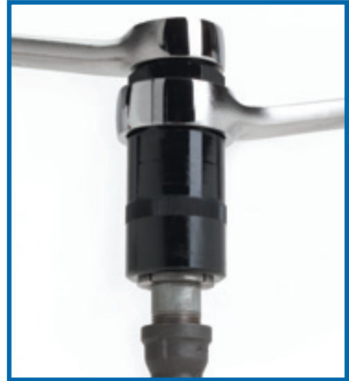
The Tight-Grip Nipple Tool in use. One wrench holds the housing in place while the other wrench turns the top nut, clamping the collet and housing assembly onto the nipple. The housing, collet, and nipple then turn as one.
